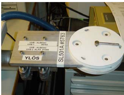
Fig3. The holder designed for the two SL501.
