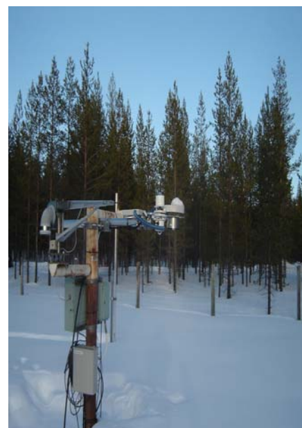
Fig5. SL501 snow UV albedo measurements in 2007.
