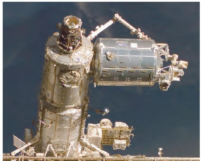
Figure 4. Mounting of SOLAR outside of COLUMBUS.
