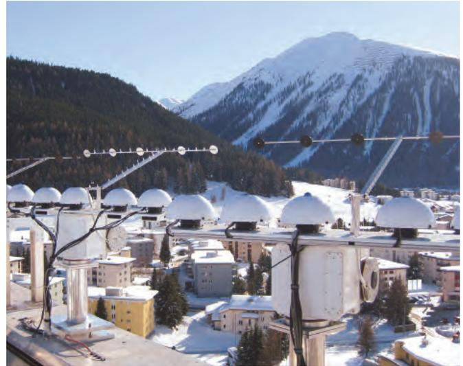
Figure 1. The roof platform of WRC-IRS with the three INTRA trackers allowing state-of-the-art pyrgeometer calibrations using shading disks.
