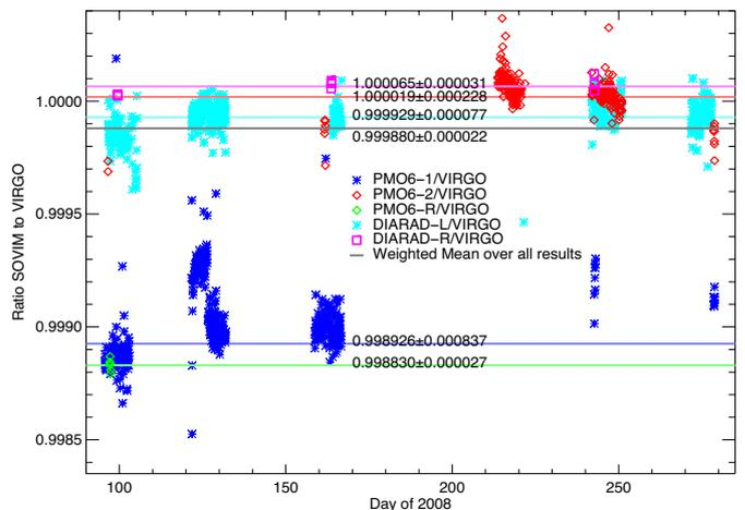
**Figure 2.** Ratio of the irradiance measured by SOVIM and determined from VIRGO. The overall weighted mean ratio is with  $0.99988 \pm 0.00002$ , and the results from the SOVIM radiometers are only 120 ppm below the one of VIRGO.
