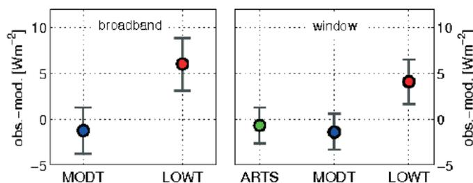
**Figure 1.** Errorbars indicating mean and standard deviation of observed minus modeled DLR of 40 clear-sky night situations at Payerne using various band parameter models. ARTS and MODTRAN calculations are within the measurement uncertainty of  $\pm 2\text{ Wm}^{-2}$ , whereas LOWTRAN is outside.
