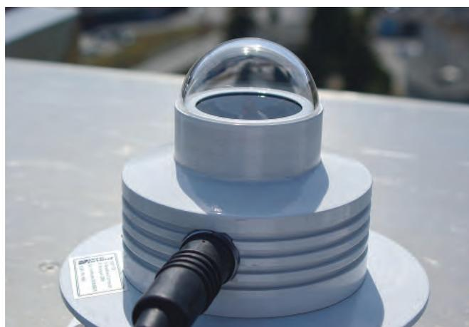
**Figure 1.** A Solar Light 501 UV broadband Radiometer is designed to measure erythemally weighted UV irradiance. The calibration procedure for such instruments was adapted, to convert the output signal to UV irradiance weighted with different UV response functions.
