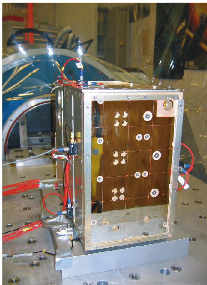
**Figure 1.** Hardware built at PMOD/WRC is tested for space qualification. The PREMOS instrument is mounted on the vibration test adapter at the University of Berne. The red cables connect the various 3-dimensional accelerometers to acquire the response of the PREMOS structure during vibration.
