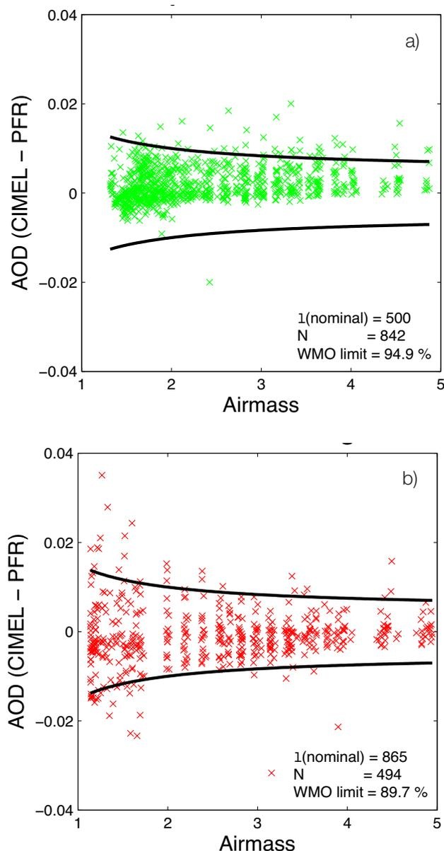
**Figure 1.** CIMEL-PFR AOD difference versus airmass, illustrating the WMO criteria for traceability (solid line) at: a) Ispra Sept. 8-26, 2008 ( $\lambda = 500$  nm), and b) Cabauw June 11-12, 2008 ( $\lambda = 865$  nm).
