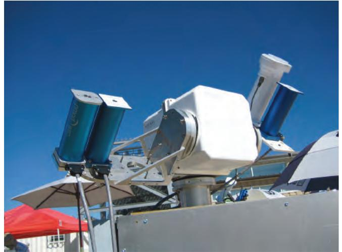
**Figure 1.** At the US National Pyrheliometer Comparisons the WRR-calibrated transfer instruments AHF-32455 (right, top) and PMO6-0401 (right, bottom) share a solar tracker with two other PMO6s.
