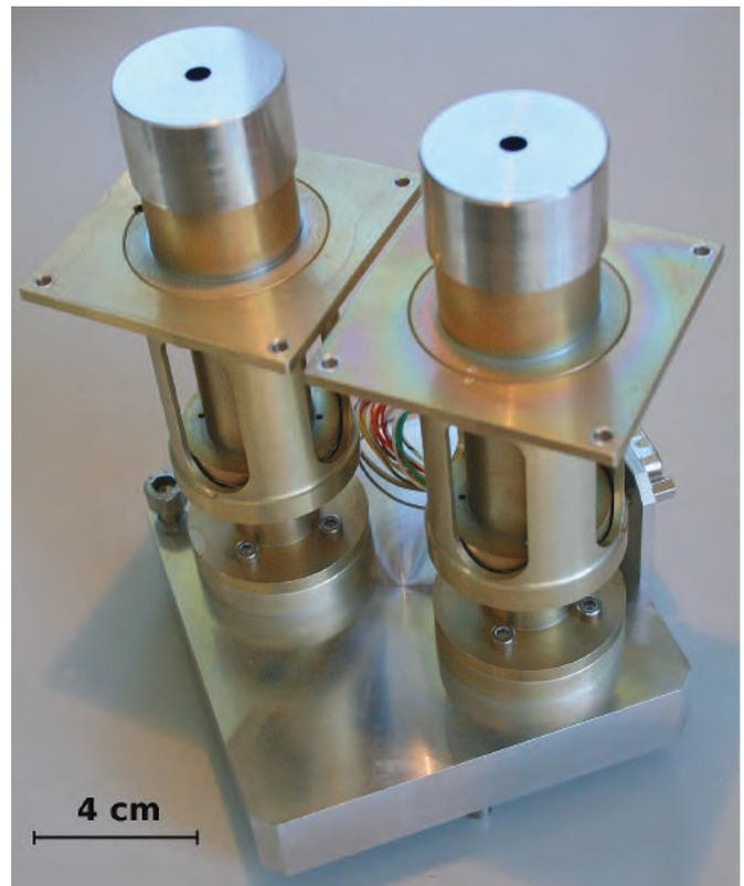
**Figure 2.** The dual cavity monitor MITRA prototype. Not shown is the instrument housing which acts as a wind-shield and thus makes it insensitive to ambient temperature.
