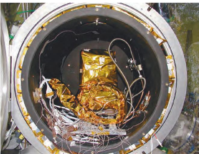
**Figure 1.** PREMOS Thermal Balance Test. The experiment is placed in a vacuum chamber and wrapped with MLI (Multi-Layer Insulation). Several temperature sensors are placed on different locations of the instrument to provide measurement points for verification of the thermal model.
