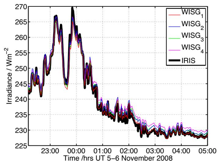
Figure 3. Downwelling longwave irradiance measurements from November 5 to 6, 2008. The IRIS radiometer is shown by the thick black line while the WISG pyrgeometers are shown by the thin colored lines.
