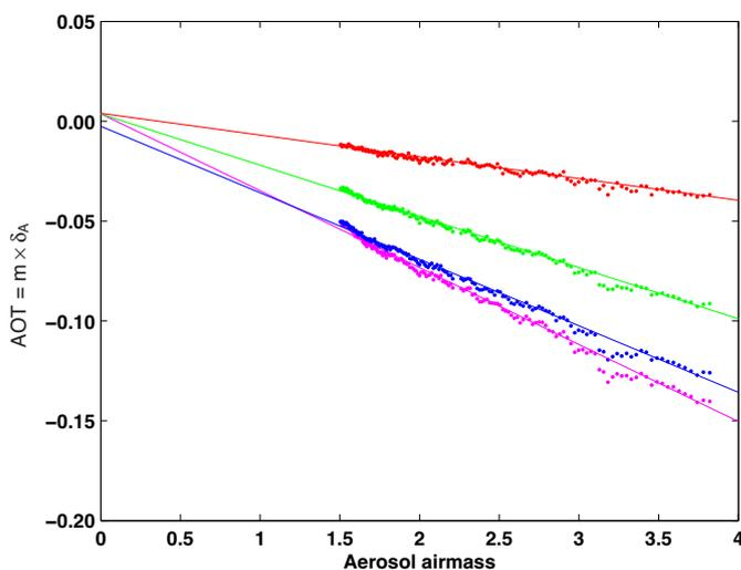
**Figure 1.** Selected Langley extrapolation for N26 on 16.07.2008. Regression lines match exoatmospheric optical depth within 0.004 or EAV within 0.4%.
