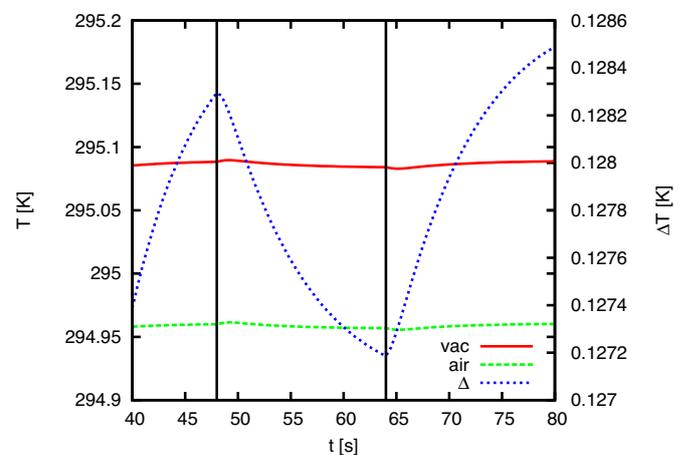
**Figure 1.** Thermal simulations of the temperature at the cavity base. The air-vacuum difference (dotted line) is representative of the non-equivalence of radiant and electrical heating. When the shutter period is ~30 seconds the spurious error signal due to non-equivalence is phase-shifted by 90° with respect to the shutter cycle and hence maximally suppressed by the phase-sensitive signal analysis (shutter switches are indicated by the vertical lines).
