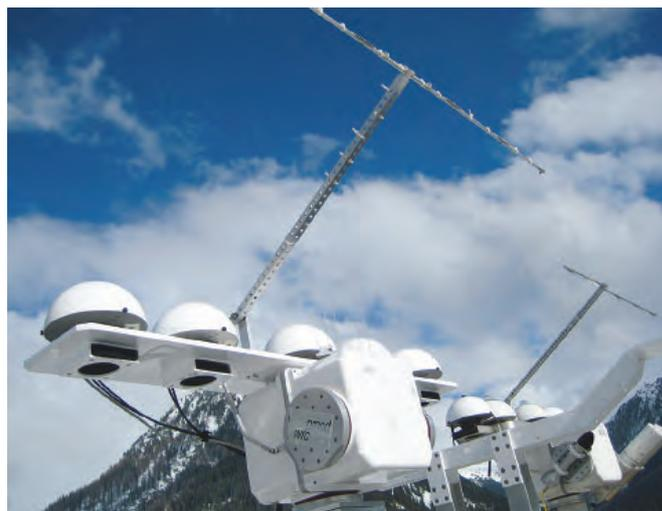
**Figure 1.** The new BRUSAG sun tracker in operation on the roof of the PMOD/WRC building.
