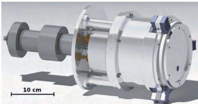
**Figure 1.** The CSAR instrument without vacuum tank. The dark gray part on the left is the cryogenic cooler which allows the instrument to be cooled to 20 Kelvin.
