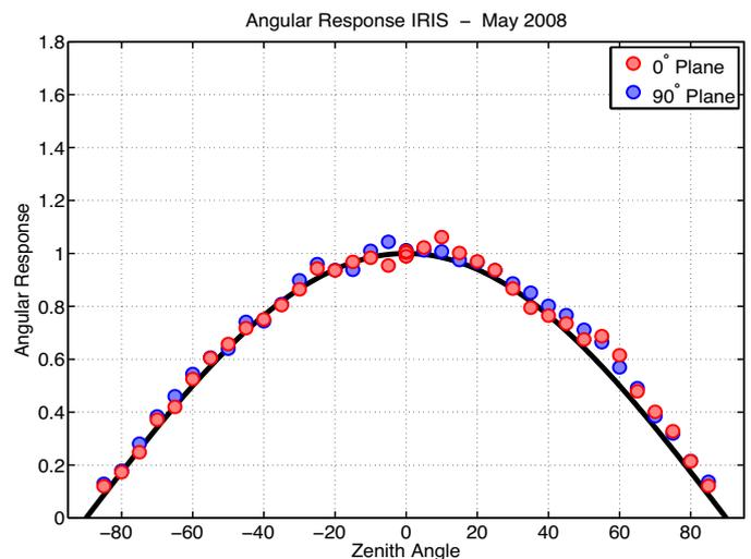
Figure 2. Angular response of the IRIS radiometer in two planes. The nominal cosine response is shown as the thick black line.
