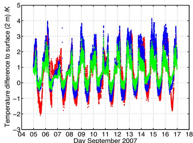
**Figure 1.** Air temperature from pyrgeometer measurements (red curve), 30 m (blue) and 10 m (green) temperature from the tower relative to synoptic temperature at Payerne.
