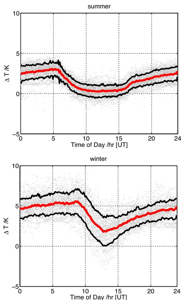
**Figure 2.** Diurnal course of ABL temperature derived from pyrgeometer measurements for summer (top) and winter (bottom) at Davos. Mean and standard deviation are highlighted in red and black, respectively.
