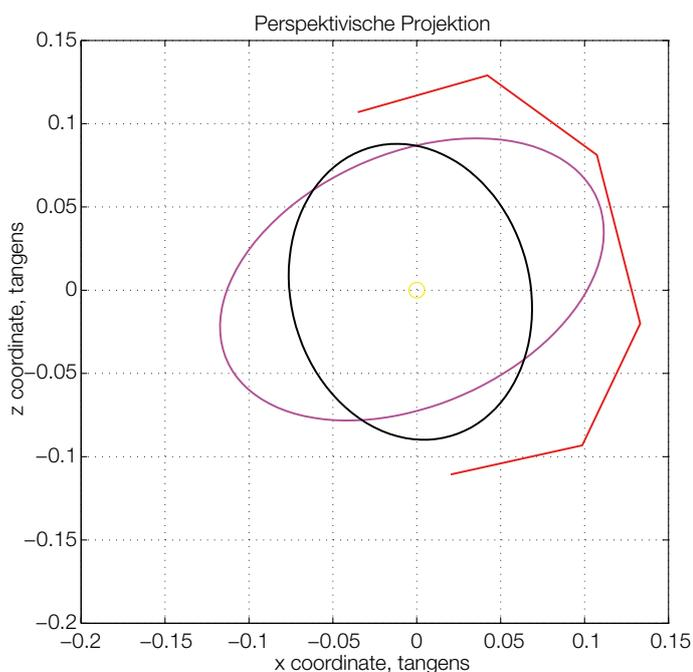
Figure 3. Field-of-view as seen from the laboratory. The black ellipse is the primary mirror and the pink ellipse is the secondary mirror. The yellow circle in the middle of the graph represents the sun with a diameter of half a degree.
