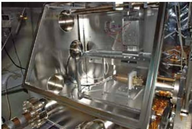
Figure 1. The PREMOS/PICARD absolute radiometer mounted on a motorized translation stage inside the TRF vacuum chamber at the Laboratory for Atmospheric and Space Physics in Boulder CO.
