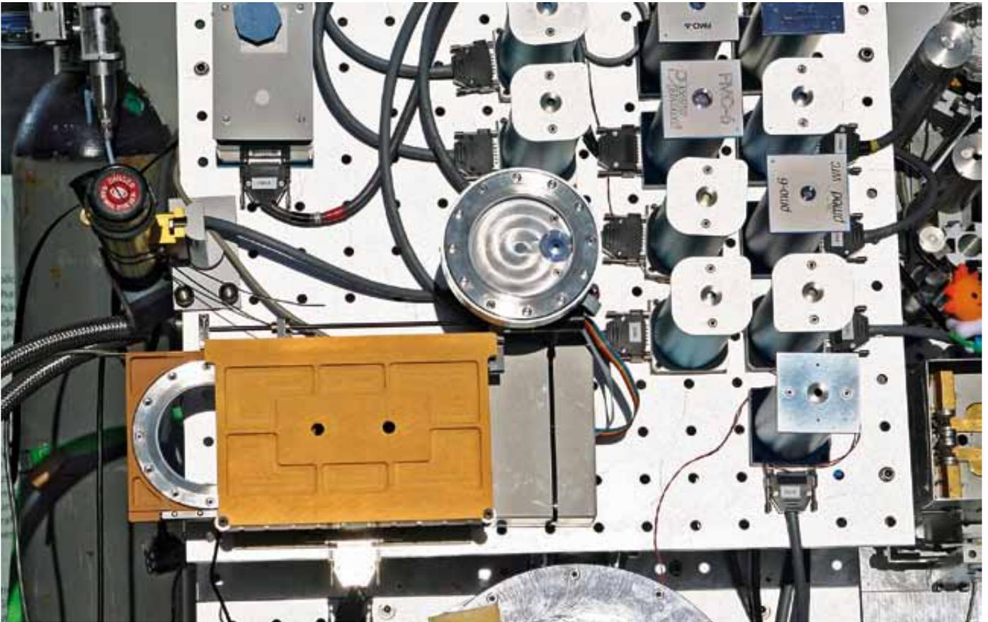
Figure 3. The Nickel-coated (brown) MITRA instrument is operated alongside CSAR on the tracking platform in Davos. A translation stage is used to move the window to the desired position.
