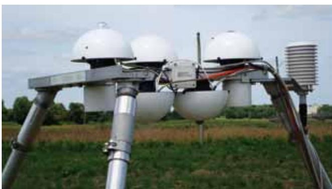
Figure 1. Instrumental setup of PMOD/WRC with two pyranometers, three pyrgeometers and Rotronic temperature and humidity sensor.
