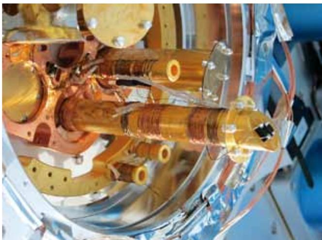
*Figure 1. The long cylindrical CSAR detector cavities have different lengths. Electrical resistors (black blocks) are used to substitute optical with electrical power. Thermal disturbances of the measurements can be avoided by wrapping the wires, which lead to the detectors, around an object on every temperature stage.*
