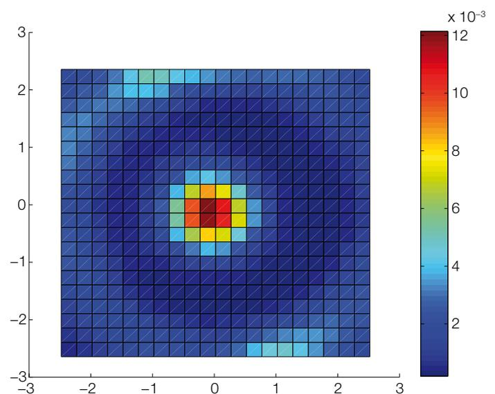
Figure 4. Absorptance map of the DARA cavity C. Yellow/red areas have a lower absorptivity than blue/green areas.
