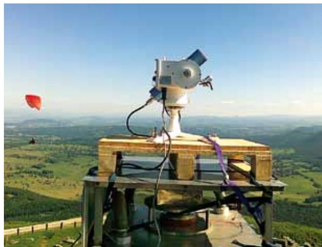
Figure 1. Temporary installation of the travelling standard PFR during an EUSAAR station audit at Puy de Dome (France).
