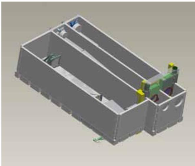
Figure 6. CAD Model of EUI Structure.
