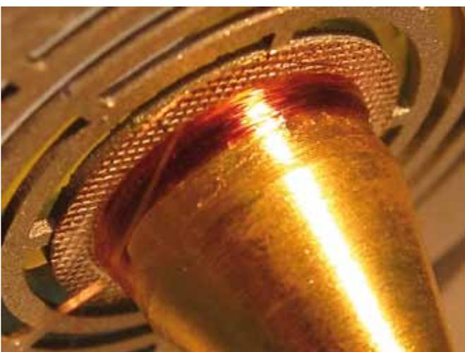
Figure 3. Copper coil thermometer glued to a MITRA detector. The amount of applied glue is hard to control which affects the thermal capacity of the detector.
