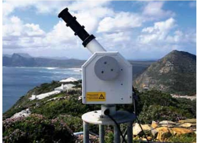
*Figure 1. PFR at Cape Point, South Africa. View towards the North showing the marine location. The black baffle tube protects the window from contamination by mineral dust and salt spray under high wind conditions.*
