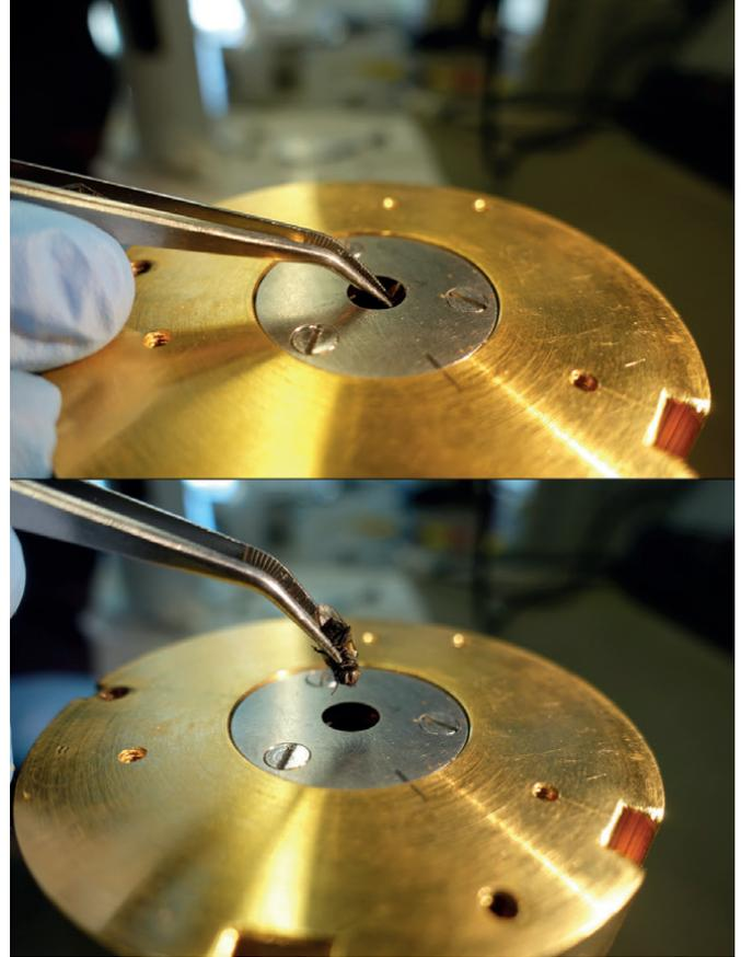
Figure 1. A dead insect was removed from the sensor cavity of the WSG pyrhemometer, HF18748, restoring its original sensitivity on 28 February. The procedure required extreme care to avoid scratching the delicate edge of the radiometric aperture.
