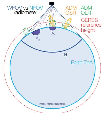
Figure 2. Schematic illustration (not to scale) of the different radiation fields of the terrestrial outgoing radiation as observed with a WFOV (dark blue lines) and NFOV (violet lines) radiometer (from Haberreiter et al., in preparation).
