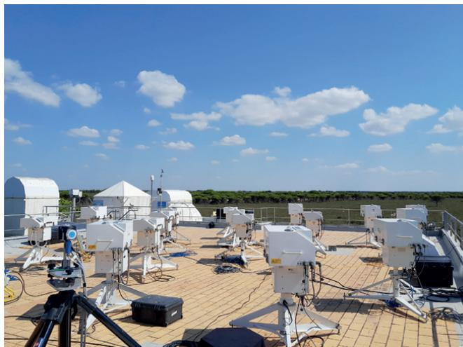
Figure 2. The 18<sup>th</sup> RBCCE inter-comparison at El Arenosillo (Spain) was conducted with 16 Brewer spectroradiometers and the QASUME reference spectroradiometer, mounted on the tripod seen in the lower left corner.
