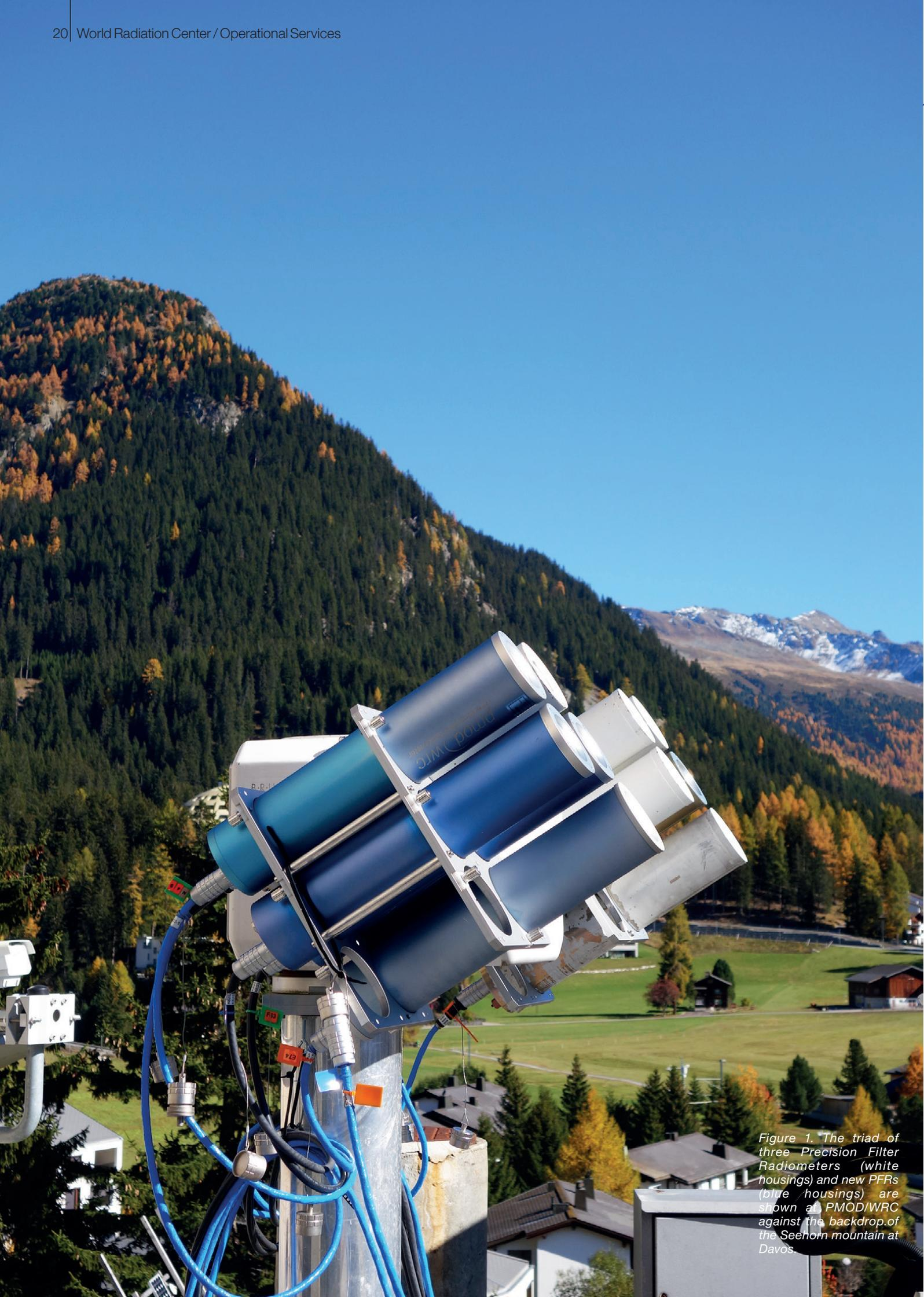
Figure 1. The triad of three Precision Filter Radiometers (white housings) and new PFRs (blue housings) are shown at PMOD/WRC against the backdrop of the Seehorn mountain at Davos.
