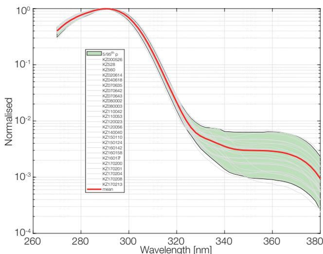
Figure 1. Spectral response function from 26 UV-S-ET radiometers (Kipp & Zonen).
