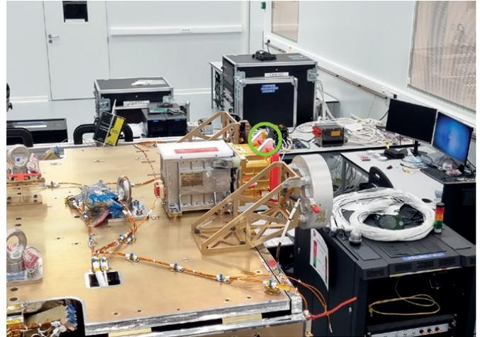
Figure 1. DARA mounted on the PROBA-3 occulter spacecraft. The green circle highlights the laser trackers for instrument alignment.
