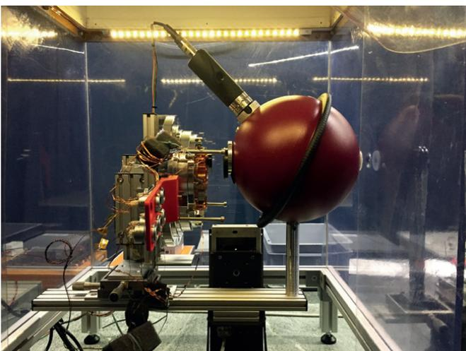
Figure 1. Installation of the CSAR detector head (on the left) together with the integrating sphere (on the right) inside the flow box in the optical laboratory at PMOD/WRC.
