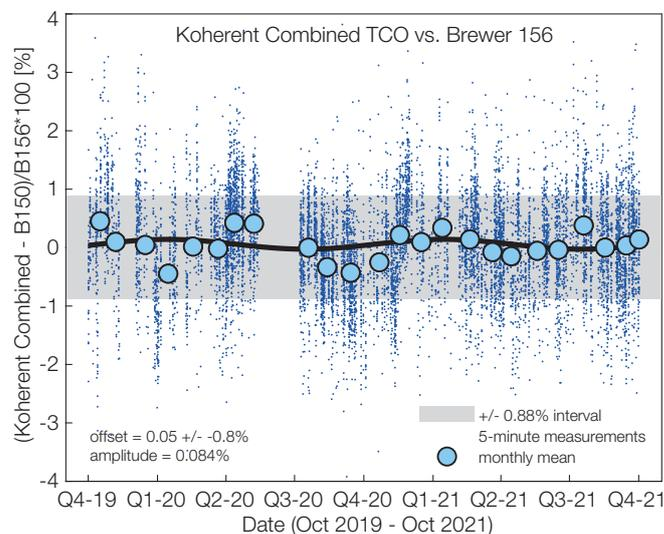
Figure 2. Relative difference between Koherent (LSF and CDR combined) and Brewer 156 double monochromator. The small blue points indicate the synchronised measurements with five minute intervals. The light blue circles are monthly means. The grey area indicates the standard deviation of the relative difference between the three retrievals used for the combined product. The seasonal amplitude is 0.084% with a long-term offset of 0.05%.
