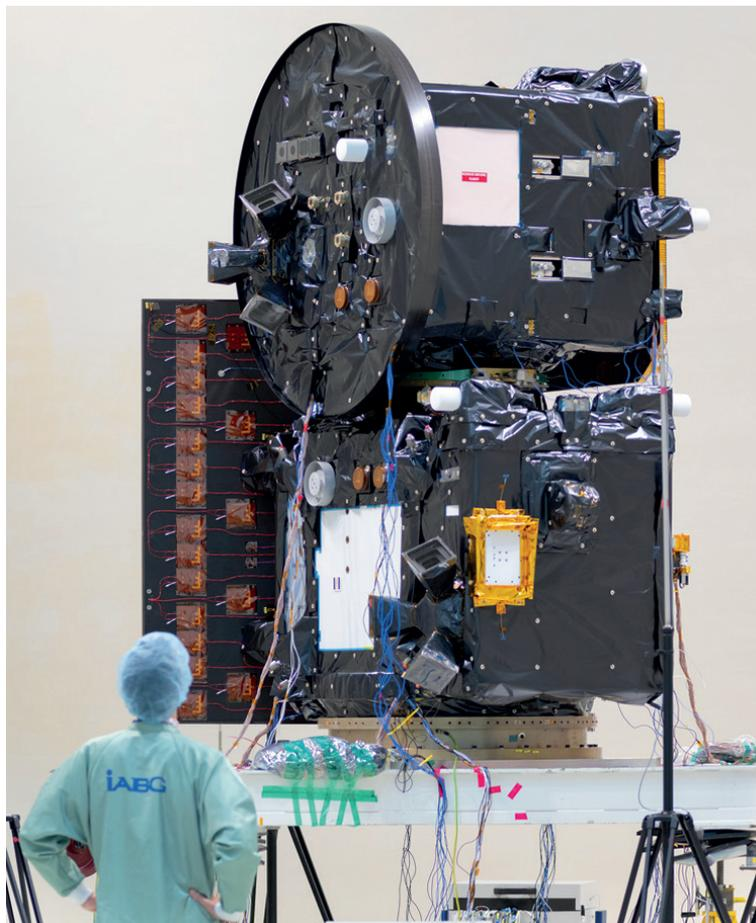
Figure 2. The combined PROBA-3 stack, with the Occulter satellite on top of the Coronagraph satellite, seen during environmental testing at IABG in Germany. (Image: courtesy of ESA)
