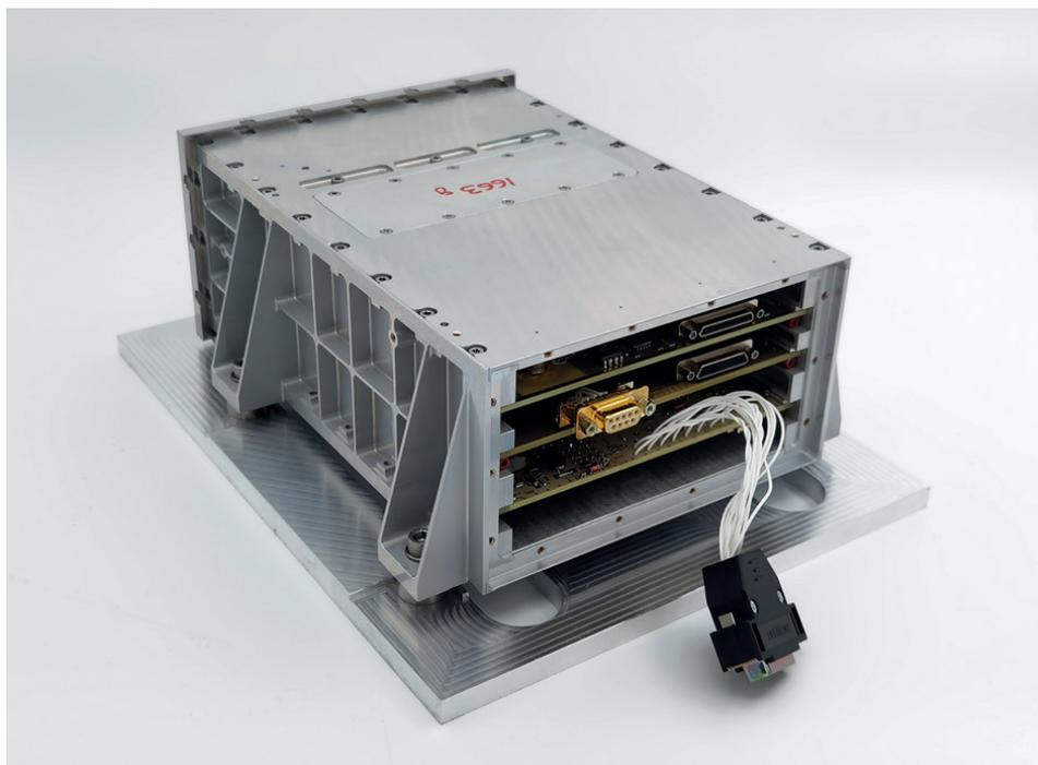
Figure 8. The SoSpIM Engineering Model.
