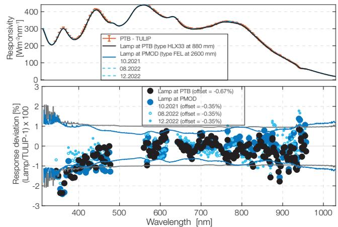
Figure 2. PSR#009 irradiance responsivity based on TULIP calibration and lamp-based calibrations at PTB and PMOD/WRC (upper panel). Normalised deviations of the lamp and laser-based calibrations (lower panel). The grey and blue lines represent the relative expanded uncertainty of the PTB and PMOD/WRC calibration setups, respectively.
