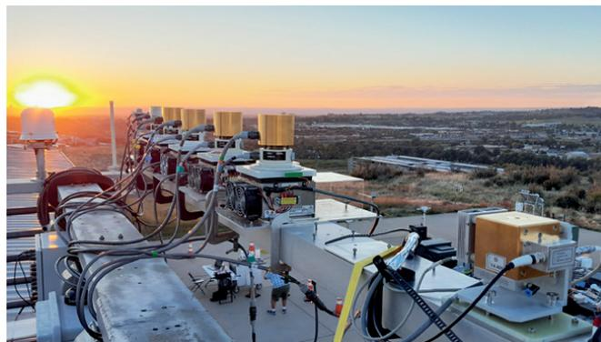
Figure 2. Absolute Cavity Pyrgeometers (ACPs) and an Infra-Red Integrating Sphere (IRIS; in the foreground) on the roof of a measurement platform during the NREL Comparison of ACPs, IRIS, and pyrgeometers traceable to the World Infrared Standard Group. The campaign ran from 25 September - 6 October, 2023, in Golden (Colorado, USA).
