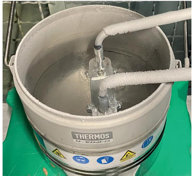
Figure 7. Setup using liquid nitrogen for thermal cycling of adhesive samples to cryogenic temperatures.
