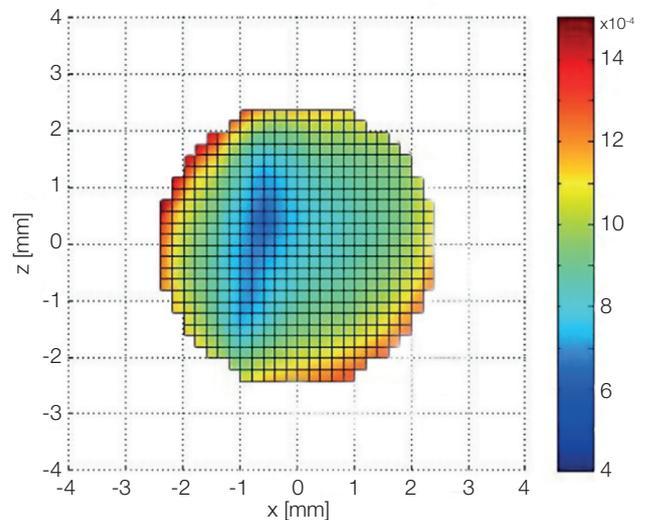
Figure 2. Reflectivity map of CSAR cavity at 532 nm showing the reflectivity distribution over the cavity area. The map was obtained during the test run using a Carbon Nanotubes reference sample S-VIS from Surrey Nano Systems Ltd., and shows preliminary results.
