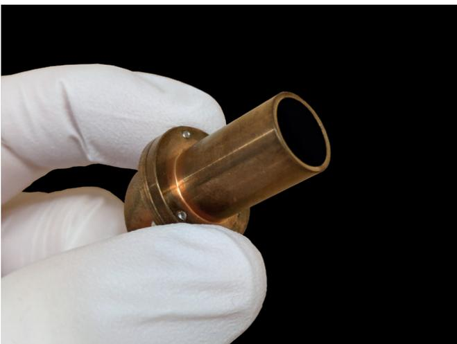
Figure 6. A 99.99% black CSAR cavity coupon with carbon nanotube coating.
