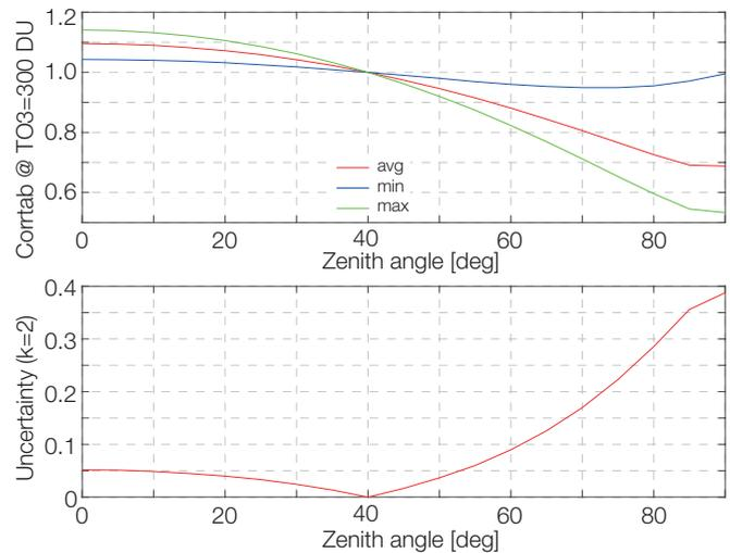
Figure 2. Average spectral mismatch correction function for UV-S-ET radiometers (Kipp & Zonen) as a function of the solar zenith angle (upper panel) and its associated uncertainty (lower panel).
