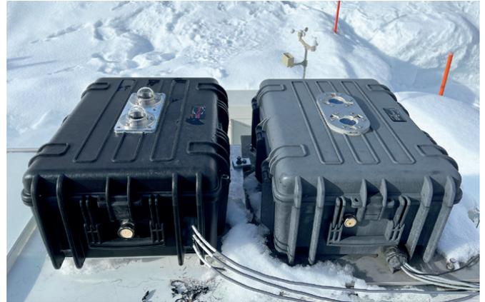
Figure 2. Housings of the two LuxMeters on the roof of the Dobson container.
