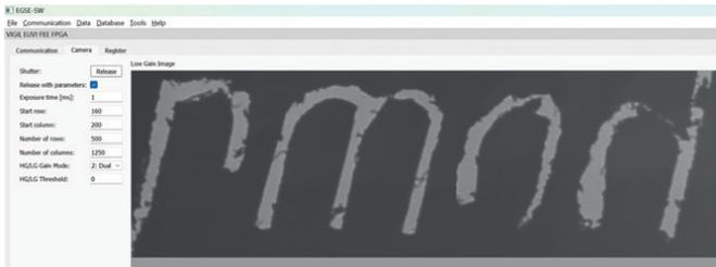
Figure 5. First successful readout of the CMOS image detector.
