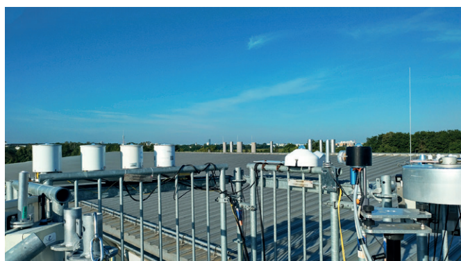
Figure 1. The QASUME site audit to BFS (Munich, Germany). The inter-comparison campaign lasted from 3 May to 7 June 2024. The data from three of the four BTS spectroradiometers (left) were compared to Qasume. It's entrance optic can be seen on the right of the picture.
