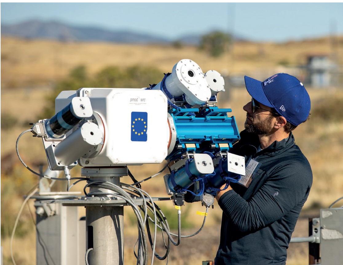
Figure 1. The WRC-SRS technician is installing the four travelling standard group pyrheliometers on the mobile solar tracker at NREL, using the new mounting brackets. The pyrheliometers on the left belong to the German Weather Service, DWD.
