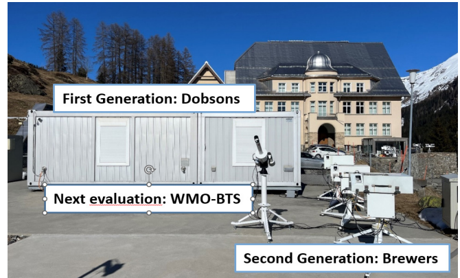
Figure 2. The WMO-BTS as guest at PMOD/WRC for comparison with first generation of TOC instruments (Dobsons in the container) and second generation of TOC instruments (Brewers).
