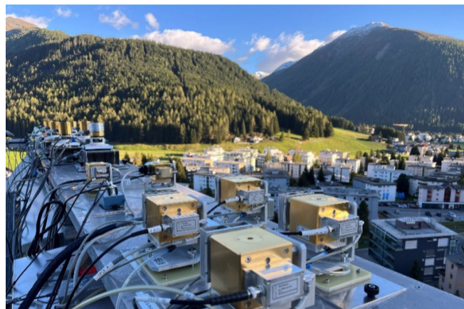
Figure 2. Measurement platform on the roof of PMOD/WRC with IRIS radiometers in the front and ACP radiometers in the back.
