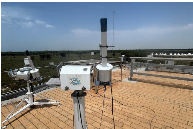
Figure 1. The BTS from Davos on a sun tracker at the regional Brewer intercomparison 2025 in Spain.
