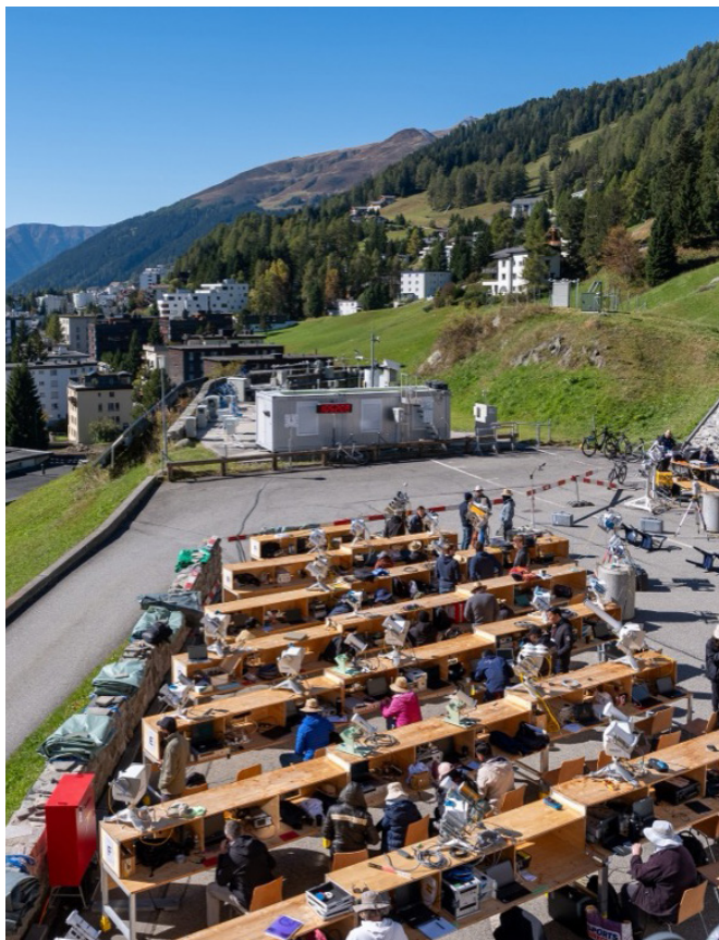
Figure 1. Participants of the 14th WMO International Pyrheliometer Comparison are collecting solar irradiance measurements during excellent weather conditions on October 2nd. Acoustic signals and a reference clock on the measuring field ensure strict adherence to the prescribed sequence and timing of the measurements, which is necessary for accurately comparing them to the reference values from the World Standard Group (WSG)
